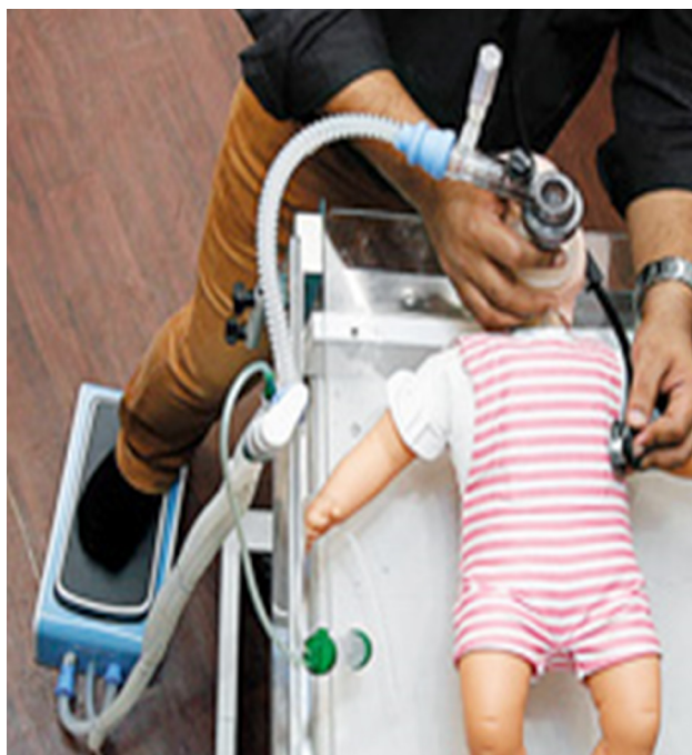
Figure 1 NeoBreathe novel foot operated resuscitator.
