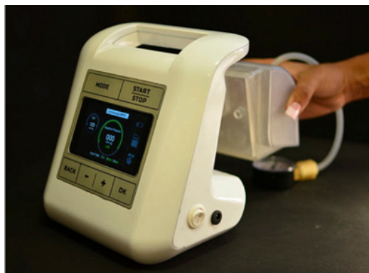
Fig.1: The NPWT device developed by Inochi Care Private Limited, New Delhi, India, was used in the present study. It consists of a suction pump unit capable of generating a continuous vacuum of 40-200 mm Hg and a disposable, transparent 500 ml capacity canister for collecting the wound exudates.
